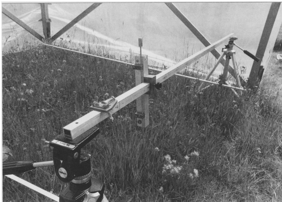
Fig. 2. Point quadrat apparatus used for the present study.
