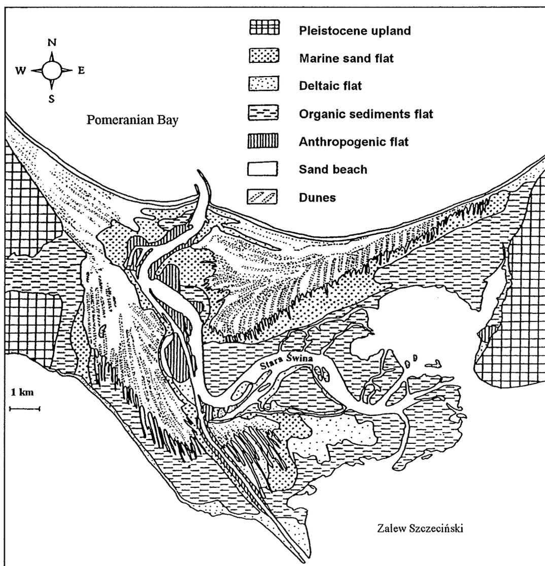
Fig. 31. Geomorphologic map of the Świna Barrier (after Matkowska et al. 1977, modified).
