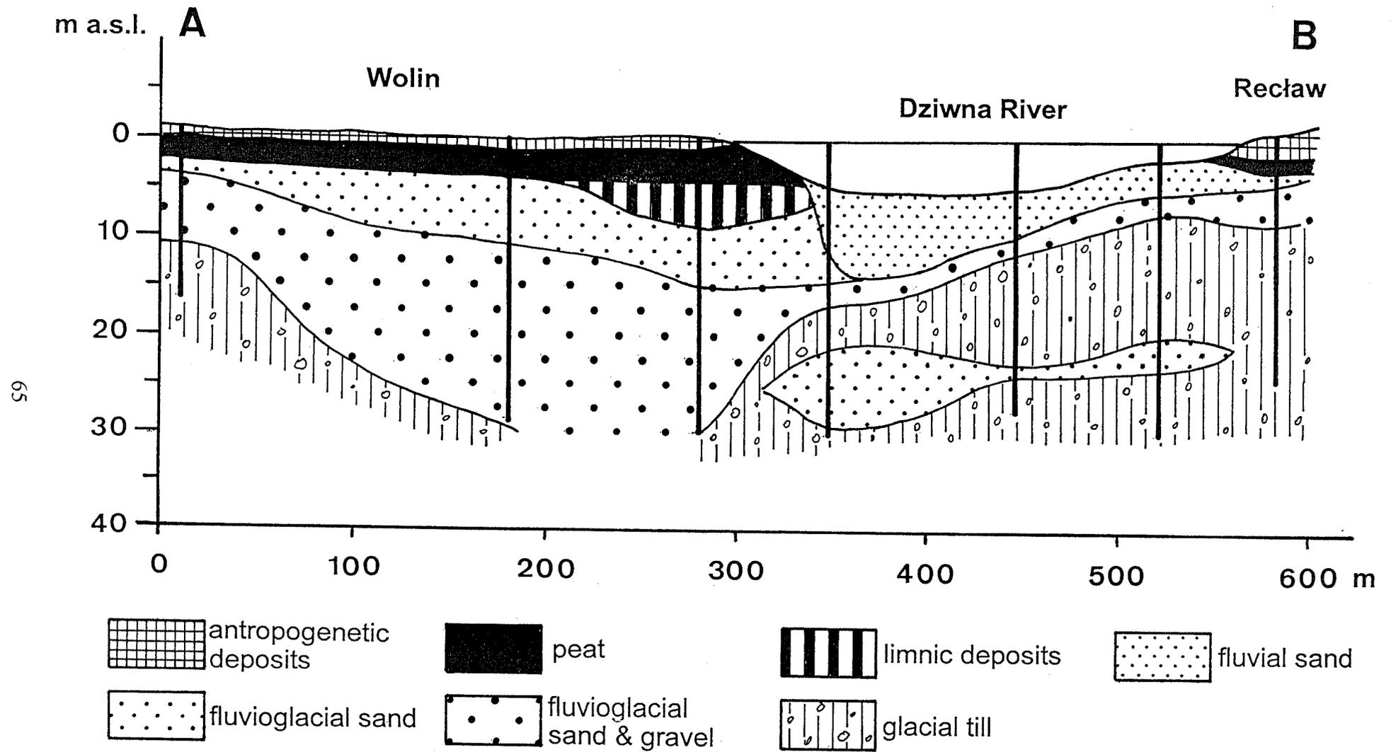
Fig. 35. Cross-section of the Dziwna valley between Wolin and Reclaw
